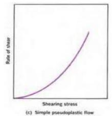
Furthermore, because no part of the curve is linear, the viscosity of a pseudoplastic material cannot be expressed by any single value. The viscosity of a pseudoplastic substance decreases with an increasing rate of shear and this system is known as a shear thinning system.
