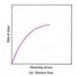
Dilatant behavior can be explained as follows. At rest, the particles are closely packed with minimal inter-particle volume (voids). The amount of vehicle in the suspension is sufficient, however, to fill voids and permit particles to move relative to one another at low rates of shear. Thus, a dilatant suspension can be poured from a bottle because under these conditions it is reasonably fluid.
